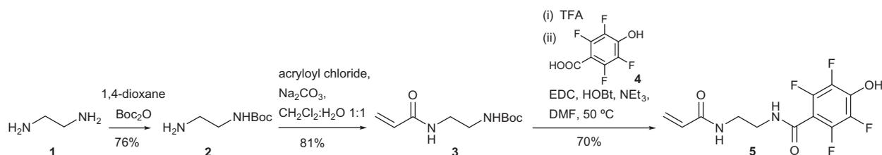
**Scheme 1.** Synthesis of the TFP (TetraFluoroPhenol) acrylate monomer unit (5). TFA = trifluoroacetic acid, Boc = *tert*-butoxycarbonyl, EDC = 1-(3-dimethylaminopropyl)-3-ethylcarbodiimide hydrochloride, HOBT = 1-hydroxybenzotriazole.
