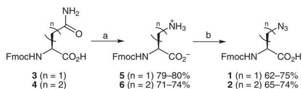
**Scheme 1** Reagents and conditions: a) [Bis(trifluoroacetoxy)iodo]benzene, DMF–H<sub>2</sub>O (2:1), pyridine, 14 h; b) imidazole-1-sulfonyl azide hydrochloride, K<sub>2</sub>CO<sub>3</sub>, H<sub>2</sub>O–MeOH–CH<sub>2</sub>Cl<sub>2</sub> (1:1:1), pH 9, 18 h.
