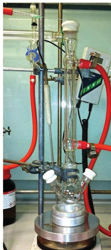
Figure 6 | Equipment setup for Grignard formation (Step 3).
