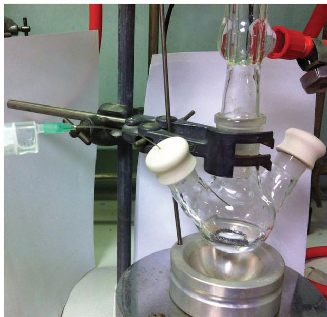
Figure 8 | Transfer of anhydrous THF into the reaction vessel (Step 5).
