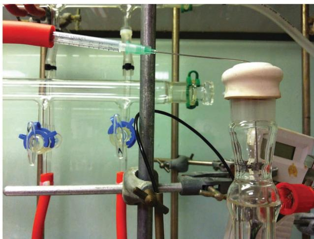
Figure 7 | Close-up of attachment of reaction system to dual nitrogen-vacuum manifold (Step 3).
